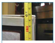
Most refrigeration door gaskets are 4 sided, but when you are working with large walk in cooler doors, you will find many of those are 3 sided gaskets with no bottom. If the gasket is NOT 4 sided, then you will need to specify which sides you would like us to include. Typically on 3 sided gaskets the bottom is a door sweep.
